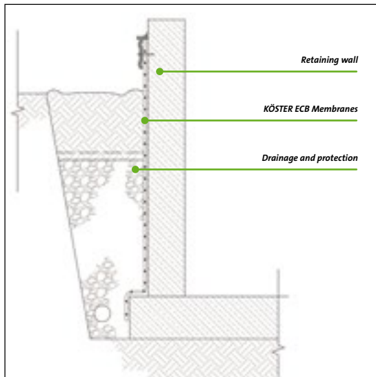
In situ retaining walls
