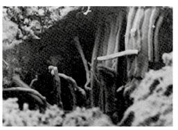
The cristallization of the salts in the pores of the KÖSTER Restoration Plaster prevents the salts from causing damage.
