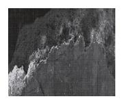
Electron microscope scan: White areas: latent hydraulic compounds which penetrated into the pore structure of the substrate - and reacted to form a a pore blocking crystal.
