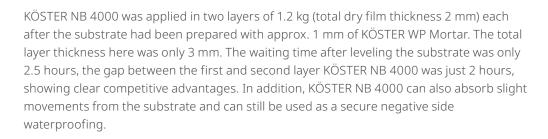
KÖSTER WP Mortar has also passed the test requirements according to WTA. The mortar showed its full performance from a dry layer thickness of just 4 mm.
